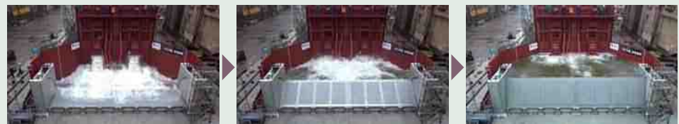
Performance of motions and watertight of the large scale "neo RiSe" is confirmed by water falling tank with 600 m³.
