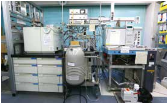
Nano EA (elemental analyzer) / IRMS (isotopic mass spectrometer) capable of measuring the smallest amounts of trace sample isotopes by this type of device worldwide
