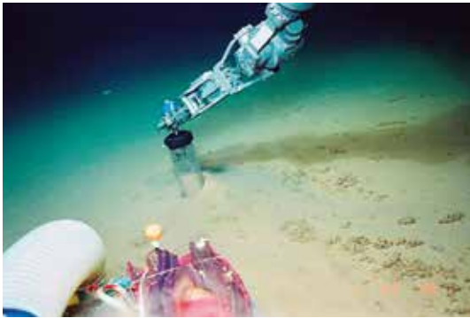
Collecting sediment from the bottom of the Challenger Deep (depth: 10,896 m) in the Mariana Trench. Our efforts will hopefully lead to the discovery of novel microbial resources.
