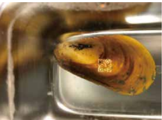
Development of deep sea organism identification technology using underwater laser processing technology
